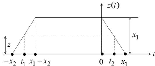
Fig. 3. The graph of changing duration of coincidence of two vehicles
