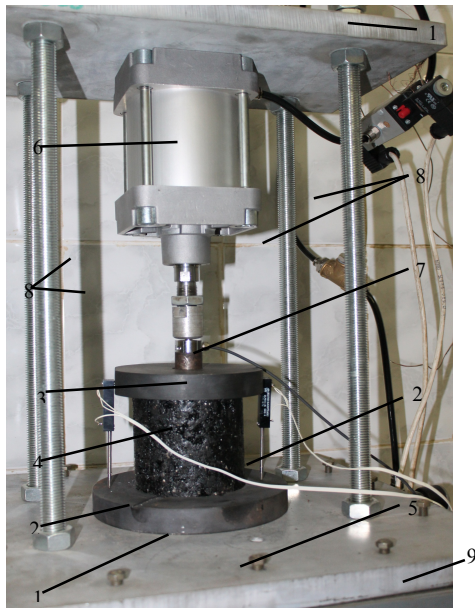
Fig. 5 – Power unit of the laboratory equipment for testing asphalt concrete: 1 – asphalt concrete sample; 2 – sensors of motion; 3 – sensor of force; 4 – pressure foot; 5 – bearing foot; 6 – pneumatic cylinder; 7 – tip; 8 – supporting bars; 9 – lower base plate; 10 – upper base plate
