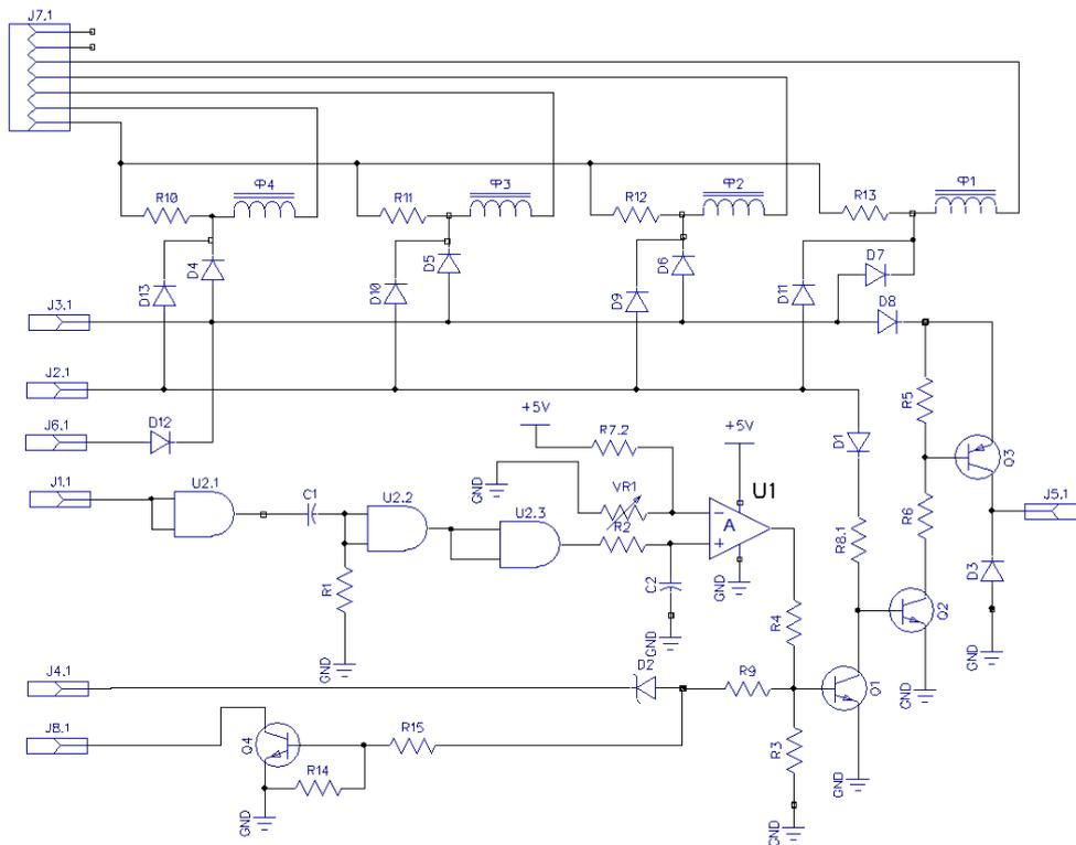
Fig. 3. Schematic diagram of the system start-stop hybrid vehicle conversion after conversion
