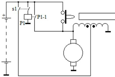
Fig. 2. The additional force P1 relay starter for start-stop system
