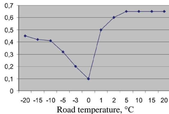
Fig. 1. Effect of road temperature on grip coefficient [12]
