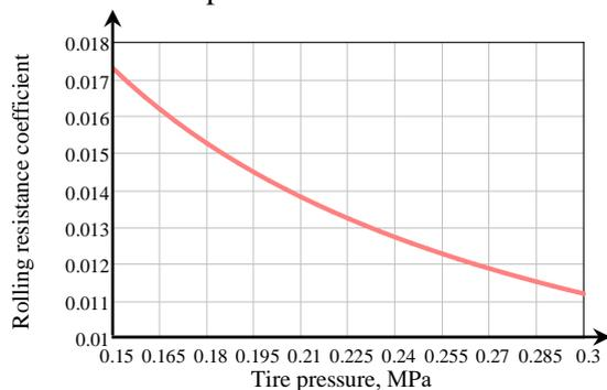
Fig. 5. The dependence of the coefficient of rolling resistance on the internal pressure of the gas filler in the tire
