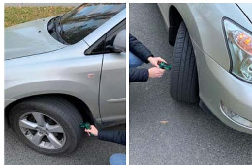
Fig. 3. Measurement of temperature in the tread and shoulder zone using a non-contact thermometer
