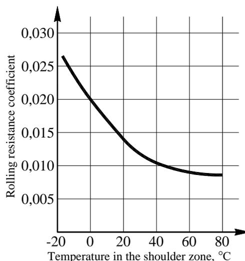
Fig. 7. The dependence of the coefficient of rolling resistance on the temperature in the shoulder zone [13]
