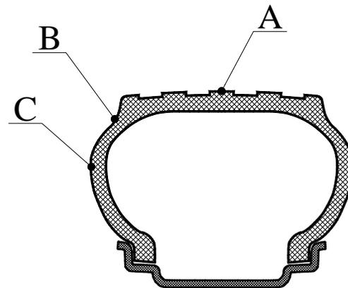
Fig. 2. Points at which the surface layer temperature was measured
