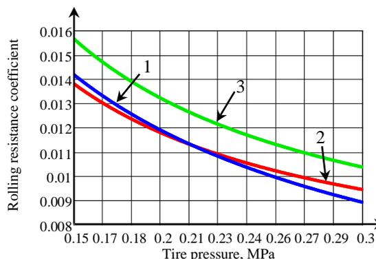
Fig. 6. The dependence of the rolling resistance coefficient on the internal pressure of the gas filler in the tire: 1 – without taking into account the load on the wheel; 2 – wheel load 2500 H; 3 – wheel load 4000 H
