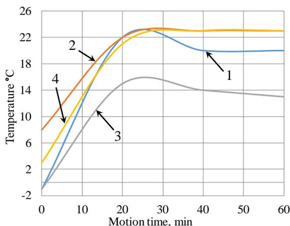
Fig. 4. Graph of the change in the temperature of the surface layers in the shoulder area of the tire during the starting mode motion: 1 – 235/60R18 (summer tires) 1°C; 2 – 235/60R18 (summer tires) 6°C; 3 – 235/55R18 (winter tires) 1°C; 4 – 235/55R20 (summer tires) 1°C
