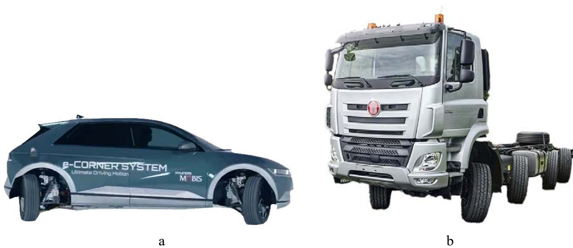
Fig. 6. Wheel steering systems: a – e-Corner system from Hyundai; b – wheel steering system from Tatra
