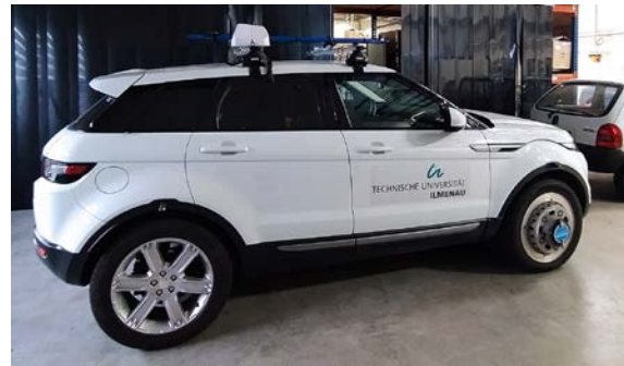
Fig. 1. The overall view of the installed external equipment on the experimental vehicle
