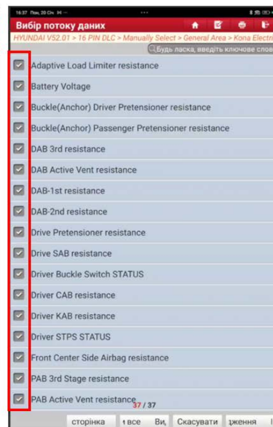
Fig. 4. Airbag ECU: a – screen for selecting the Airbag unit; b – selection of “Read Data Stream”; c – data stream screen of the Airbag unit
